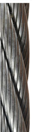
**SUPER ATLANTIC®** HEAVY COMPACTED FISHING WIRE ROPES especially designed for large pelagic trawlers, midwater trawlers and demersal trawlers. It is produced in the construction 6x K (compacted) 26 WS (Warrington Seale) in order to offer an higher grade of flexibility and a very strong abrasion resistance.
