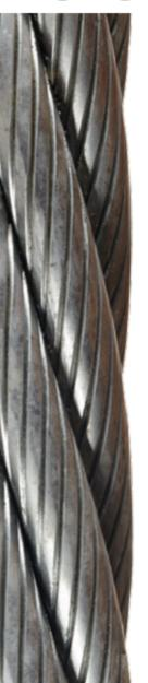
ZINCAL COMPACT® is another very successful product manufactured by OLIVEIRA SÁ. It is a compacted wire rope with the construction 6x K26WS, manufactured both with steel or fiber core. ZINCAL COMPACT® has all the wires covered with a thick lay of zinc - aluminium alloy, which gives a higher corrosion resistance to the wire rope and an improved lifetime due to this special coating.
